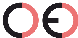
False CE Mark (too far)
